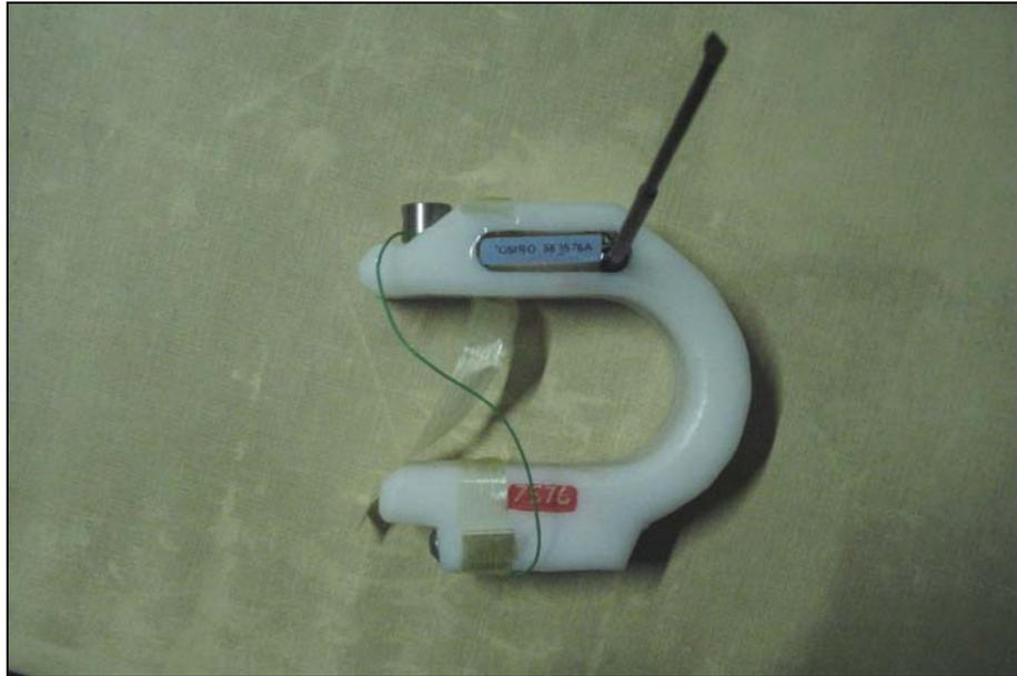
Figure 2.11. Fin tag without neoprene cover (Photos – © C. Speed).
